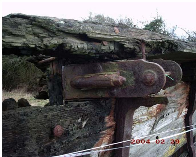
Figure 11 - One Section of the Hull Trimming Gear - Starboard Side
