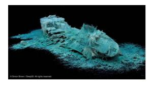
At 131m long and sitting in 32m of water the use of photogrammetry to scan the SS Thistlegorm for the Presence in the Past project presented a series of challenges. Just over 24,000 high resolution images were required to cover the ship, seabed, cargo and internal features. In the field the immediate requirement for on site image management was paramount: to reduce the risk of individual images, or a small series of images, being lost in the volume of data.
